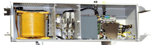
Example of integrated LRT propulsion system, <100 kg system weight
